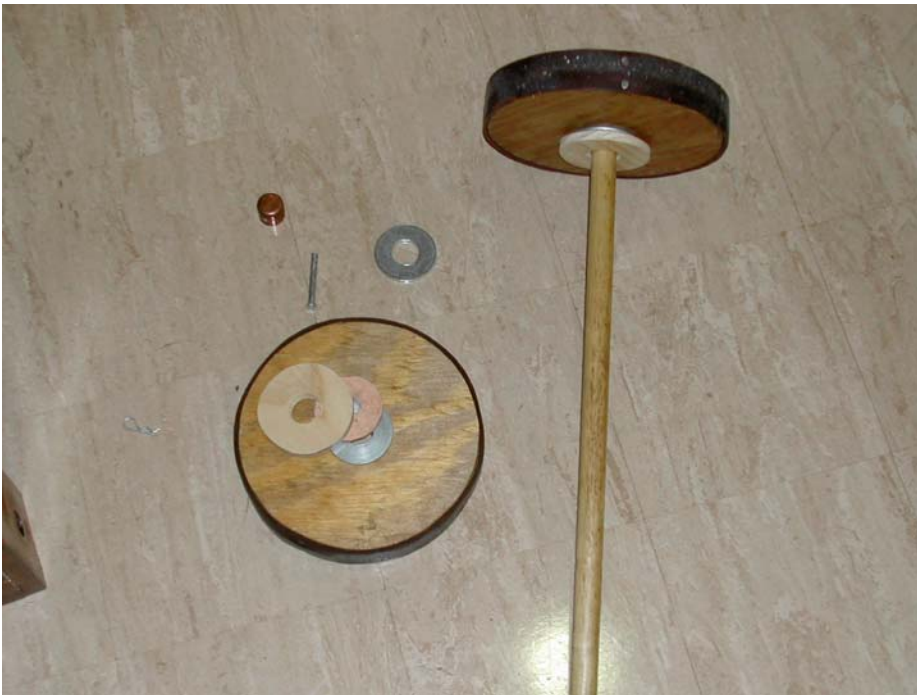
Wheel & Axle parts, wooden washers, metal washers, leather washers, cotter pins and copper caps
